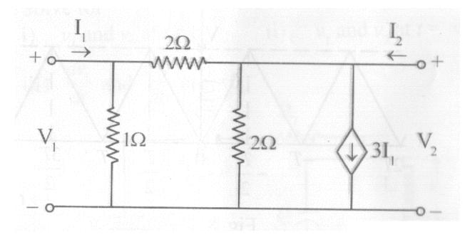
3. The circuit shown in fig. Find the ratio of V2/V1.
