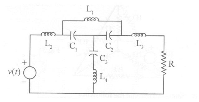
7.In the network shown in fig .determine the node voltage  $V_1AND V_2$  with respect to the reference node.
