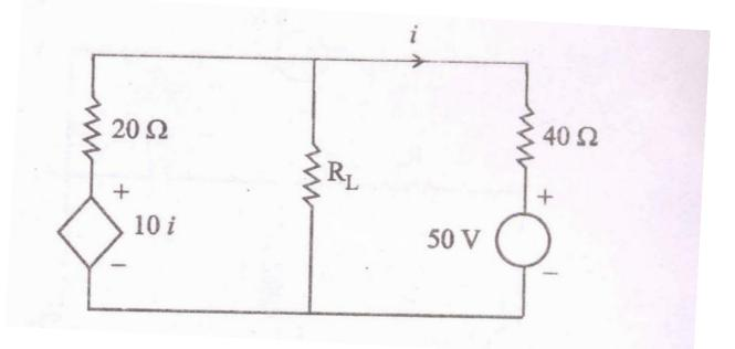
19. Calculate the current I by using superposition theorem.
